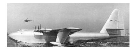
OWARD HUGHES WAS ONCE one of the richest men in America. He made millions in the aircraft industry and designed, built and flew--once--the largest aircraft ever built. That was the Spruce Goose, a flying boat with eight engines and built mostly of birch plywood. The wingspan of a 747 jumbo jet is 195 feet--the Spruce Goose is 320 feet.
